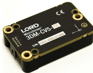
Figure 1 -3DM-CV5-15 Sensor
