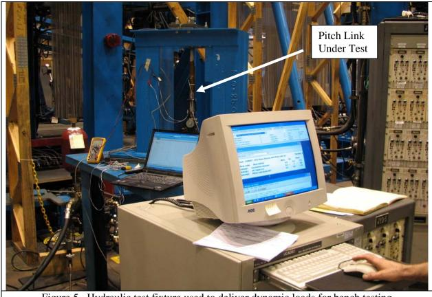
Figure 5. Hydraulic test fixture used to deliver dynamic loads for bench testing
