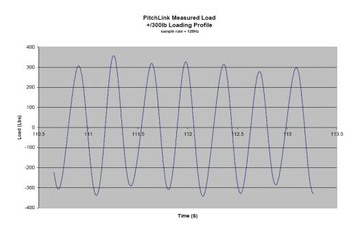
Figure 7. Load data recording from energy harvesting wireless electronics, in data logging mode (Mode 3) for Bell M412 pitch link under sinusoidal axial loading of +/- 300 lbs at ~3 cycles/sec.
