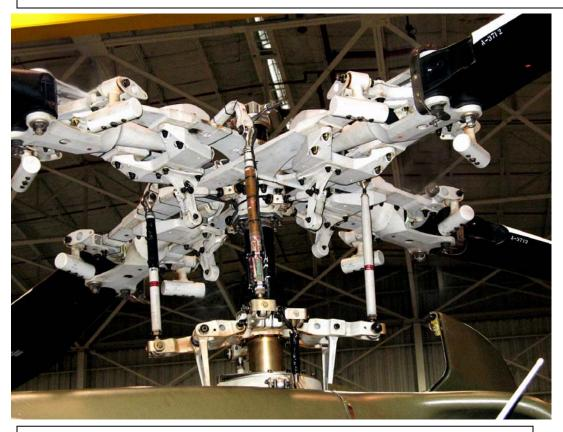
Figure 8. Energy harvesting wireless pitch link installed on Bell M412
