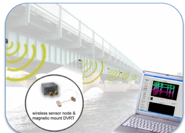
Figure 3. Scalable wireless network supports quick installation of distributed miniature sensors
