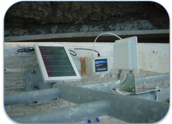
Figure 4. Energy harvesting elements enable autonomous, long-term monitoring
