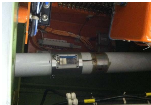
Figure 5: MQ-8B FireScout Torque-Link™ Installation
