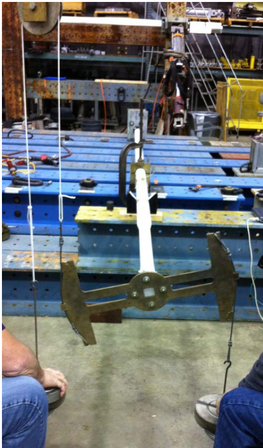
Figure 4: FireScout Torque Shaft Electronics Calibration
