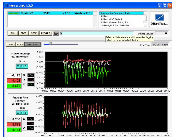
Figure 1 – Real-time, customizable acceleration and angular rate readout on MicroStrain's Inertia-Link software
