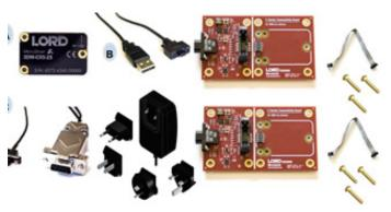
The sensor can be purchased by itself, or as part of a development kit. There are two variations of the kit.,The 3DM-CV5-10 communicates via RS232, and is only supported by the RS232 version. (p/n 6212-3010). The kit includes the C-series Connectivity Board and appropriate cables and mounting screws. This guide assumes that you have a development kit and will download the latest version of SensorConnect™ software.
