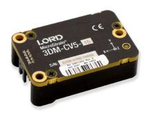
The LORD Sensing 3DM-CV5 family of industrial-grade, board-level inertial sensors provides a wide range of triaxial inertial measurements, computed attitude, and navigation solutions.
