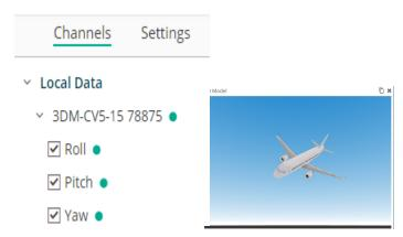
Test the linkage to the widget aircraft...pick up the sensor, and move it in 3 axes. The plane should respond.
