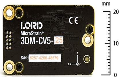
3DM-CV5-25 -miniature, industrial-grade attitude and heading reference system (AHRS) with integrated magnetometers, high noise immunity, and exceptional performance
