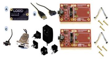
The sensor and development kit are purchased separately. There are two variations of the kit, USB (p/n 6212-3009) and RS232 (p/n 6212-3010). The C-series Connectivity Board supports both interfaces and is included in both part numbers, along with appropriate cables and mounting screws.
