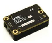
The 3DM - CV5 - 25 is an industrial- grade , board- level Attitude and Heading Reference System (AHRS) that utilizes micro inertial sensors for use in a wide range of industrial - grade applications, such as unmanned vehicle navigation, platform stabilization, and vehicle health monitoring.
