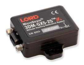
The LORD Sensing 3DM-GX5 family of high-performing, industrial-grade inertial sensors provides a wide range of triaxial inertial measurements, computed attitude, and navigation solutions.
