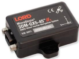
The 3DM-GX5-45 communicates through a serial connection and is monitored by a host computer. Sensor measurements and computed outputs can be viewed and recorded with SensorConnect software, available as a free download from the LORD Sensing website. Alternatively, users can write custom software with the open source data communication protocol, also available on the site. Data is time-aligned and available by either polling or continuous stream.
