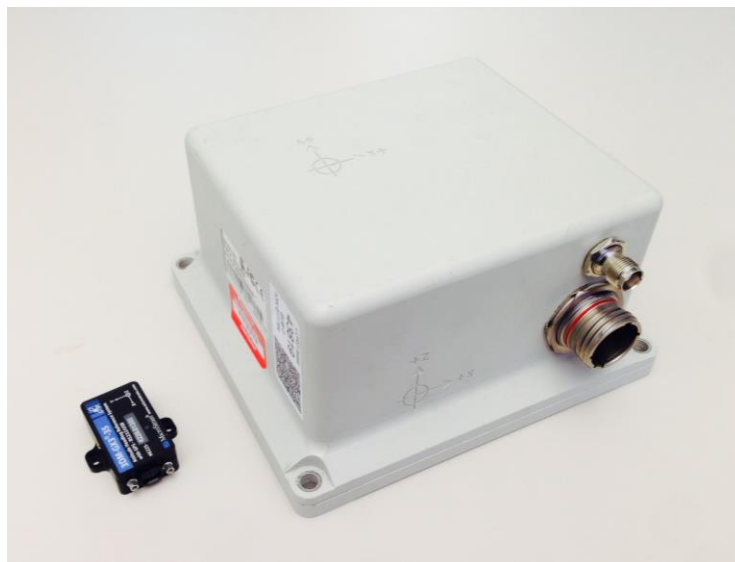
Figure 5 Photograph of GPS-INS reference unit (left) and typical Inertial Sensor under test (right).
