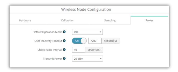
Figure 14 - Node Configuration Power Menu
