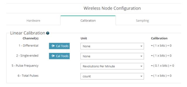
Figure 12 - Wireless Sensor Calibration Menu
