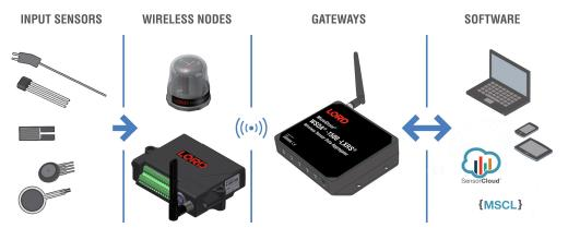
LORD Wireless Sensor Network Multiple nodes communicate through gateway using star network topology
