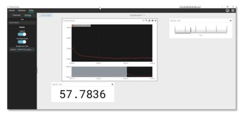
When done sampling, the node must be set to idle to communicate with it. Select Devices, highlight the node, and select the Set Nodes to Idle tile.
