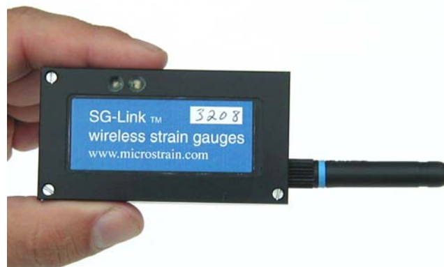
Figure 2. Compact, wireless strain sensing node with rechargeable lithium-ion battery
