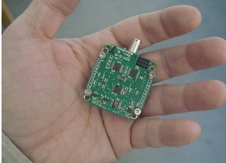
Figure 1. 3DM-GX1 Three axis orientation sensor. (Shown without enclosure.)
