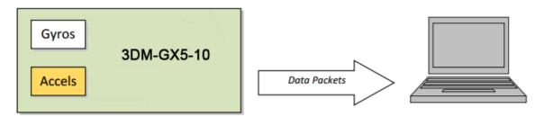
The "descriptor set" qualifier in the MIP packet header is a feature that greatly aids the management of the incoming packet stream by making it easy to sort the packets into logical sub-streams and route those streams to appropriate handlers. The first step is to parse the incoming character stream into packets.
