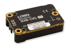
**3DM-CV5-25** – miniature, industrial-grade attitude and heading reference system (AHRS) with integrated magnetometers, high noise immunity, and exceptional performance
