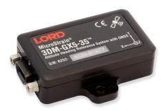
3DM-GX5-35 – miniature, high-performance, industrial-grade attitude and heading reference system (AHRS) with integrated multi-constellation GNSS, high noise immunity, and exceptional performance
