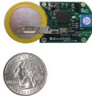
Figure 5. MicroStrain active RFID module, unpackaged, w/ battery & antenna, adjacent to US quarter.
