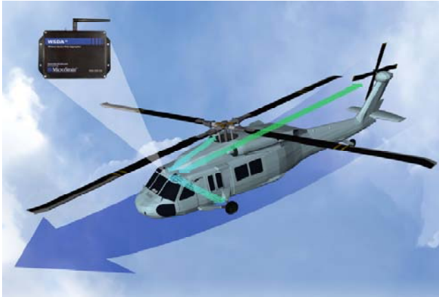
Figure 1. Wireless Sensor Data Aggregator (WSDA) collects time-stamped data from wireless/wired sensors.
