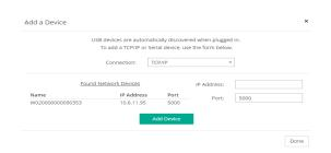
Select serial, and identify your serial port. Clicking the port select arrow should identify available comm's ports. Sensors are factory set to 115200 baud. Click Add Device, and Done:
