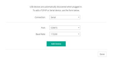
Select serial, and identify your serial port. Clicking the port select arrow should identify available comm's ports. Sensors are factory set to 115200 baud. Click Add Device, and Done:
