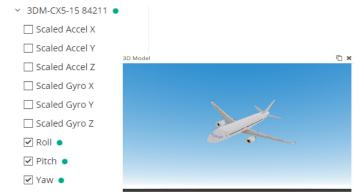
Test the linkage to the widget aircraft...pick up the sensor, and move it in 3 axes. The plane should respond.
