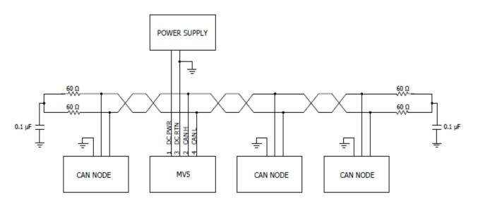
LORD recommends <u>split termination</u> on both ends of the cable for optimum EMC performance.
