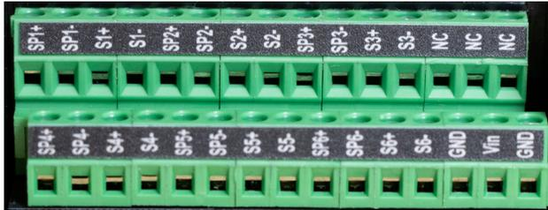
Figure 3. RTD-Link-200 Pinouts
