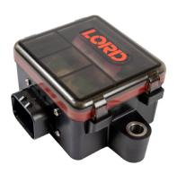
The SG-Link®-200 is a 3-channel wireless sensor with rugged, weatherproof enclosure. It includes onboard PGA, filtering, and a high-resolution ADC for precise measurement of a large range of sensor types including strain gages, load cells, pressure transducers, and accelerometers.
