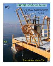
**Measurement data** was correlated between the buoy and nearest land station, validating data from the Mishmar system. The data reflects a double-peak. The first peak occurs when surface water temperature peaks, around 3 hours after peak sun.
