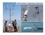
The challenge with measuring these vertical air movements on the EG-100 buoy lies with the 2-3' waves on the Dead Sea", Raanan Bodzin, GSI's lead technician, observed. "when your sensor is going up and down with the waves, the resulting air flows will be going up and down, as well. And that's where MicroStrain's 3DM-GX5-45 Inertial Navigation Sensor comes in. It allows us to remove the wave action."
