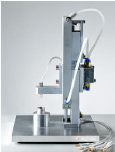
**Assembly Verification:** Employing an LVDT provides verification of proper assembly dimensions, especially when it is used in differential mode (when one sensor finds a reference surface, the other locates the part in question).
