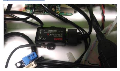
A 3DM-GX5-45 GNSS/IMU nestles away in the electronics bay of the "Tenacity" rover, with the GPS/GNSS antenna visible on the rover below.
