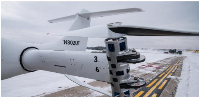
To measure revolutions, a tachometer was used. This also allowed them to produce synchronous FFT plots with the vibration sensors because the accelerometer signals could then be correlated with the phase of the propeller blade.
