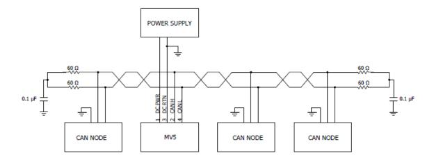
LORD recommends <u>split termination</u> on both ends of the cable for optimum EMC performance.
