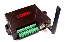
The RTD-Link\*-200 is a 6-channel wireless sensor used for precise measurement of RTDs and thermistors. No calibration is required. Select the sensor type and the node will output accurate, low noise temperature or resistance data.
