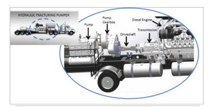
**Rigorous use conditions -** Oil and gas rigs operate in complex vibration environments . Characterizing and predicting failure of major components is key in reducing
