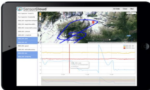
**On-site data analysis** - Using SensorCloud with MathEngine analytics tool, engineers were able to review the flight data immediately and adjust the test plan as needed.
