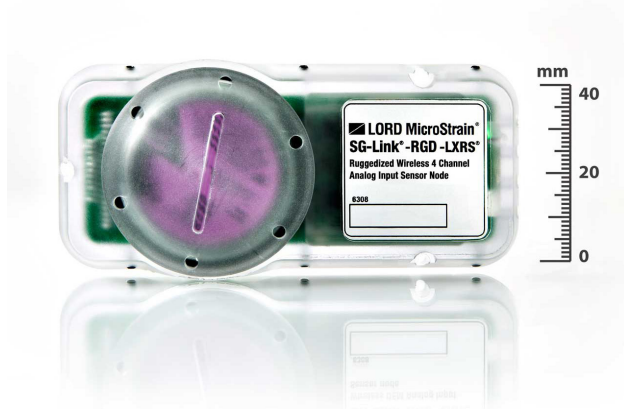
SG-Link ® -RGD-LXRS ® - versatile, ruggedized four-channel analog sensor node with integrated triaxial accelerometer
