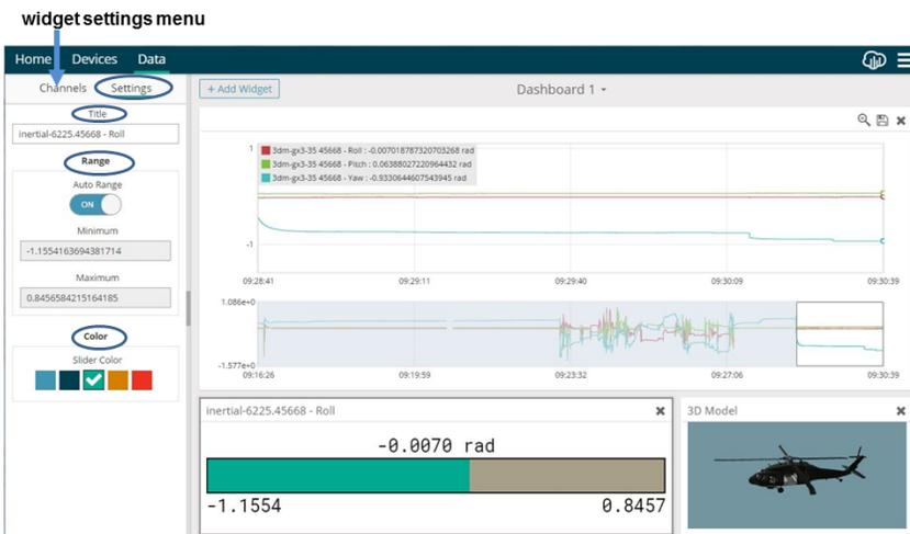
The Time Series Widget menu has two features to help optimize sensor data collection for export to a .csv file. *Snap to Latest* captures the most recent data and *Zoom* isolates specific events from a larger data sample.
